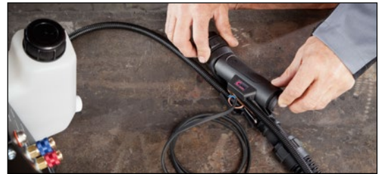
6. Lead out the flow control cable through the control cable outlet out of the housing.
